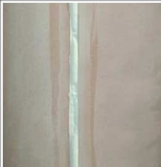
Belvorming na S_{200} -test naad 5
