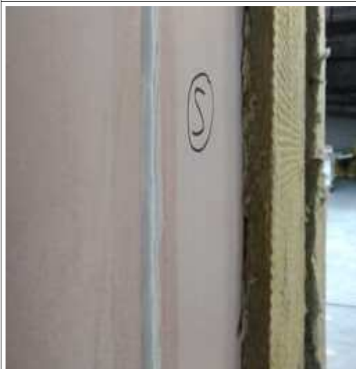
Belvorming na S_{200} -test naad 5
